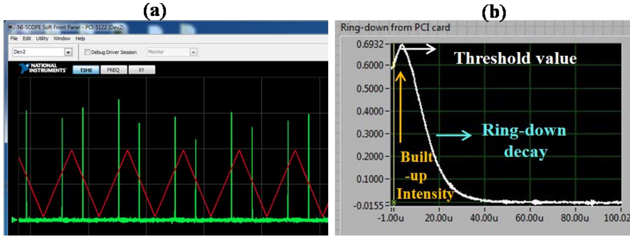
Figure 2.7 a) NI-scope image of the resonant intensity modes ( TEM_{00} ) (green) in the CRDS setup. The triangular signal (red) is the voltage applied to the PZTs for cavity length modulation. b) A typical ring-down event showing the built-up of resonant intensity up to a threshold value and the subsequent exponential decay.
